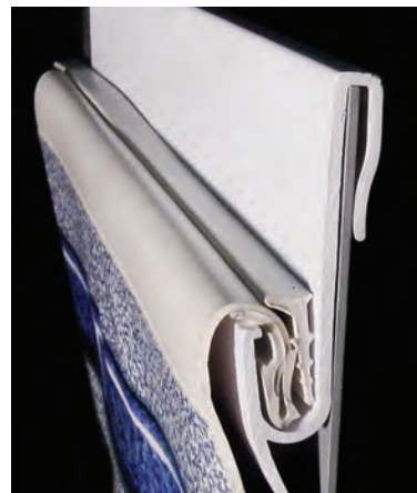
If bead receiver is too large, peel off vinyl wedge lock and insert behind liner bead to secure bead
